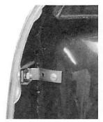
At the top of the shroud, secure a small bracket... using a 1/2" No. 12 bolt and lock nut
