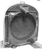
1 Position shroud on radiator with wide edge at bottom.
