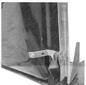
4 Attach a large bracket with a 3/4" bolt and lock nut.
