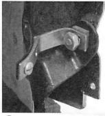
**3** At the bottom of the shroud, refasten the radiator, using a new 3/4" No 12 bolt and the existing square nut and a lock nut.
